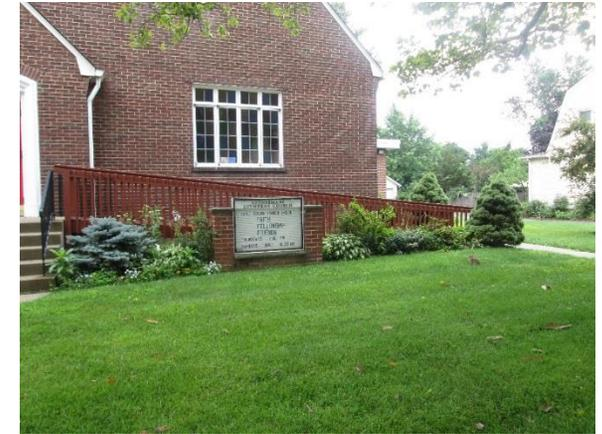
Rain gardens can be installed adjacent to the church to capture, treat, and infiltrate roof runoff by redirecting nearby downspouts. A preliminary soil assessment suggests that the soils have suitable drainage characteristics for green infrastructure.
